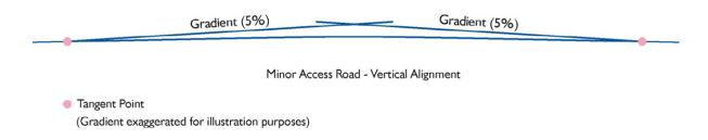
The Developer should note that side road gradients into junctions should be set at a maximum of 1:20 (5%) for the first 10m. Additionally, the minimum vertical curve length of any section of road should be not less than 20m.
