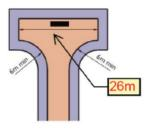
'Side T-form' turning facilities should maintain a width of 18 metres (m) and a distance of 15m from the termination of the carriageway and the start of the spur. The carriageway widths, radii and footway widths should comply with the design specification for the road which they serve.
